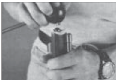
"Start" patched ball into muzzle. Figure 12-2
