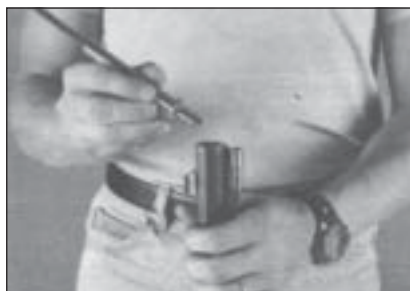
Pour measured powder charge into barrel. Figure 11-2
