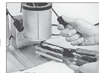
**6** Fill the mold and sprue plate so all of the sprues are connected.
