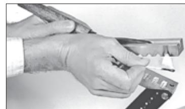
**2** Smoking the cavities with a match helps to cast better bullets. Don't use a candle as that leaves an oil film.
