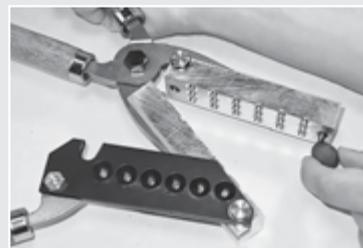
**4** Lubricate your mold using Alox Beeswax Mix Bullet Lube [Lee #90007]. **DO NOT USE Lee Liquid Alox** as it will bake on the mold surface, preventing proper closure.
