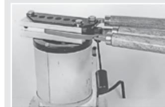
**3** Pre-heat your mold by laying it on top of your lead melter. Dip corner of mold into molten metal and hold there for 30 seconds. If the lead solidifies on the mold block, it's an indication that mold is not hot enough.
